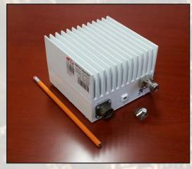
This smallest and lightest 10W(P3dB) L-To C-Band Block Up Converter is based on GaN technology. It is designed to be mounted on the feed horn. High power efficiency resulting in low current (>2 amps) .The unit covers all three C-Band sub-bands: Standard (5.85-6.425 GHz), Palapa (6.365-6.725 GHz) and Insat (6.725-7.05 GHz).
